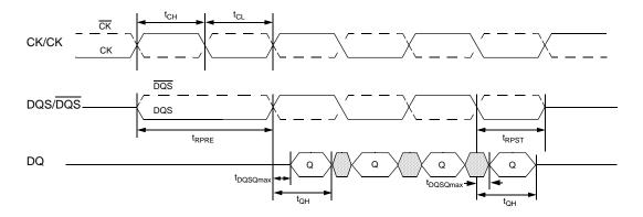
Figure -- Data output (read) timing
