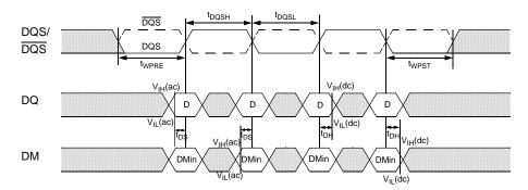
Figure -- Data input (write) timing
